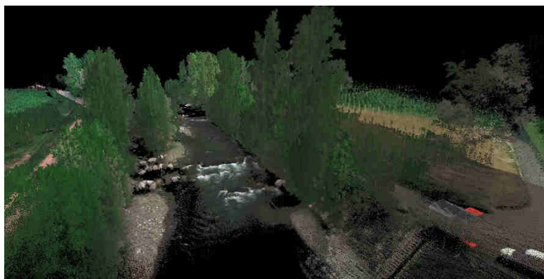
Figure 2 - LiDAR point cloud collected by RPAS survey
