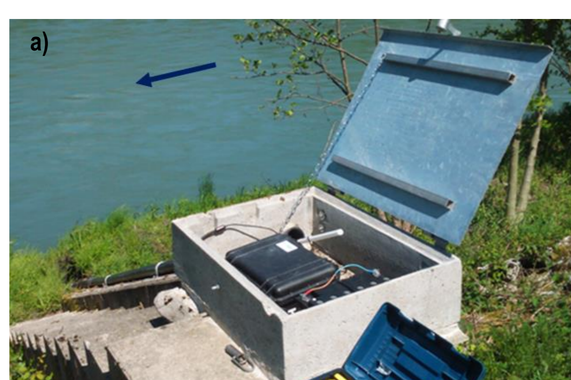
Figure 4 : Continuous monitoring from the riverside (Isère River, France) : a) the monitoring station ; b) example of temporal evolution in 2017 (time step = 1 hour)
