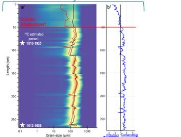
Figure 10: Core C12b - a/ Grain-size repartition; b/F1 coordinates from PCA analysis on XRF data
