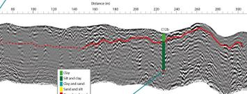
Figure 7: Ground Penetrating Radar image with cores C12a and C12b (from left to right)
