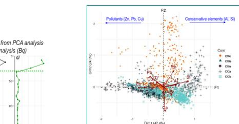
Figure 3: Principal Component Analysis on XRF data - Biplot of variables and individuals, with color varying according to sediment core
