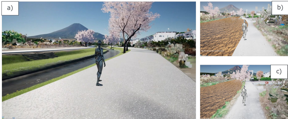
Figure 1. Digital twin for river improvement built with a game engine (Unreal engine) a) Usual situation, b) Flood time under current condition and c) under the post countermeasure condition.
