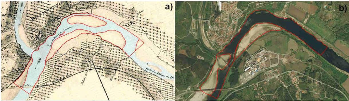
Figure 1 - Illustration of delimitation of sampling units and morphological features for Tagus (Sampling Unit 24) for the a) pre-regulation period (1898) and b) the post-regulation period (2016).
