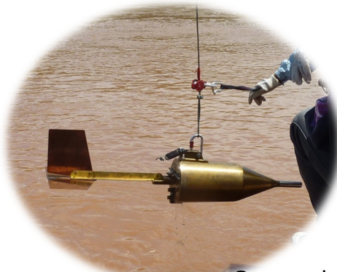
Suspended sand sampler : Delft bottle
