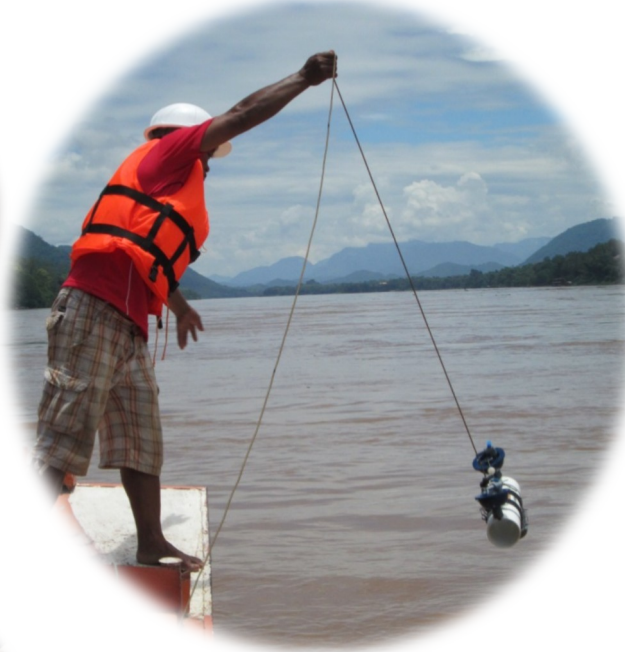
Van Dorn (Niskin) water sampler
