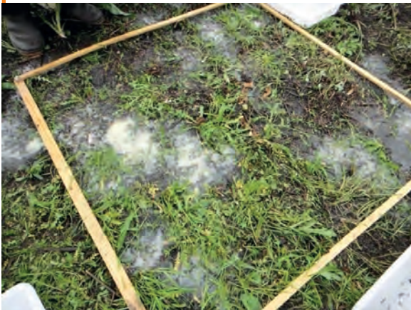
Photos 2: Quadrat of earthworm extraction using the mustard test.
