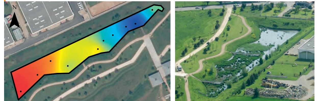
Figure 1: Distribution of water content in the Minerve infiltration basin and visualisation of the development of this flora in the Minerve basin.
