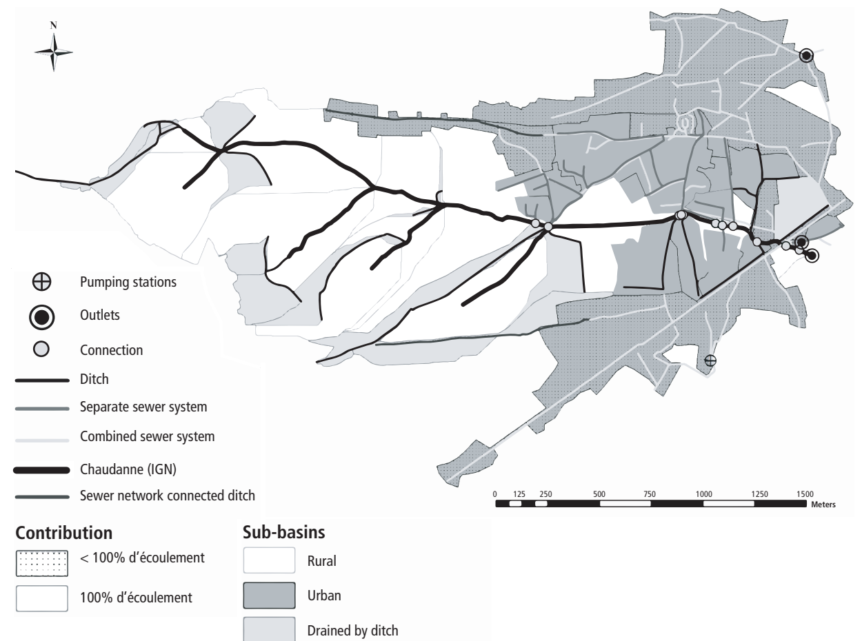
Figure 2: Final map of the Chaudanne sub-catchments and catchment boundaries under wet conditions. Urban sub-catchments are shown in dark grey, rural sub-catchments in white, and sub-catchments drained by ditches in light grey. The dotted sub-basins are only connected via CSO to the river. Subtracting the dotted areas from the basin area in wet conditions gives the basin area in dry weather (adapted from Jankowsky et al. , 2013).
