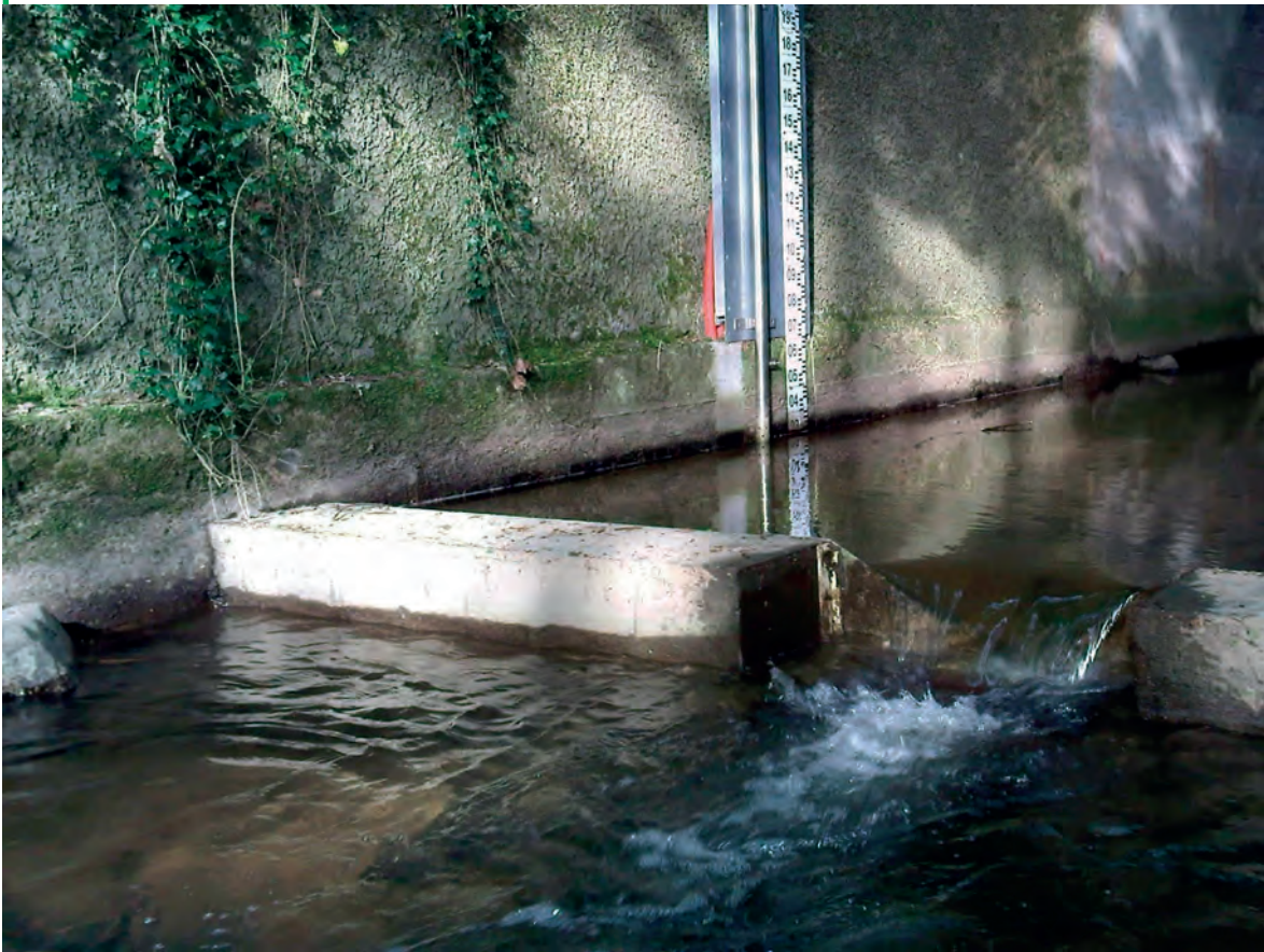
Photo 1 : Ratier hydrometric station at Saint-Genis les Ollières on OTHU site of the Yzeron catchment area. The station is equipped with a concrete weir and a triangular weir for good quality measurement of low flows (source : Mickaël Lagouy, INRAE, 2011).
