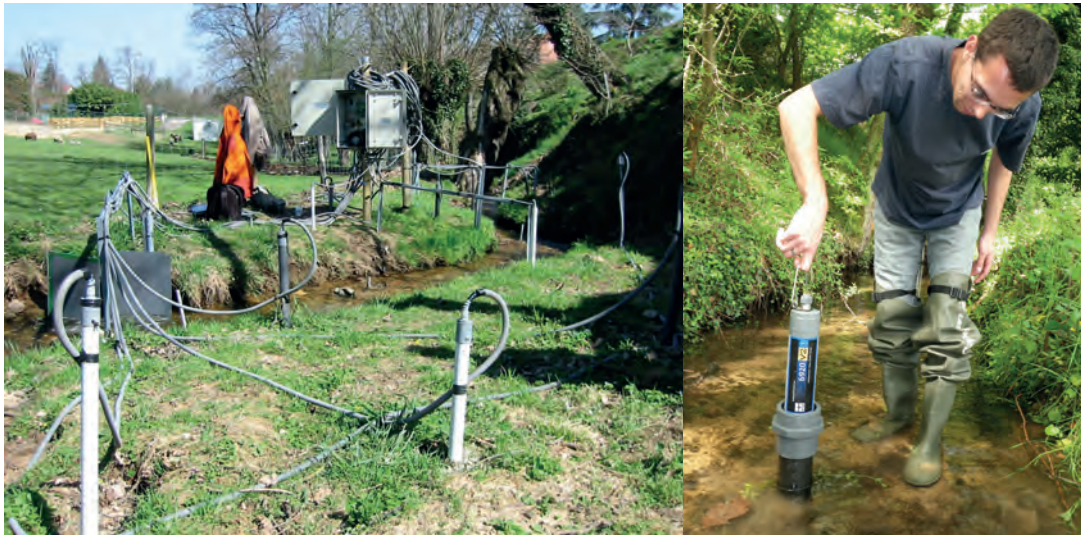
Photo 2: Taking water and fauna samples from the deep sediment, measuring exchanges between the water table and the watercourse, monitoring the quality of the water in the sediment, experimental watercourse of the Chaudanne at Grézieu-la-Varenne (source: P. Breil, INRAE, 2006).
