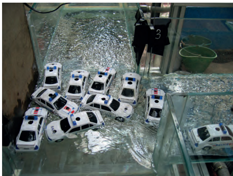
Figure 3: Modification of the flood wave by mobile obstacles: photograph of a laboratory test (top; scale 1:24) and evolution of the water depth (bottom) in the street in the absence (reference as red line) and presence of vehicles (source INSA Lyon).
