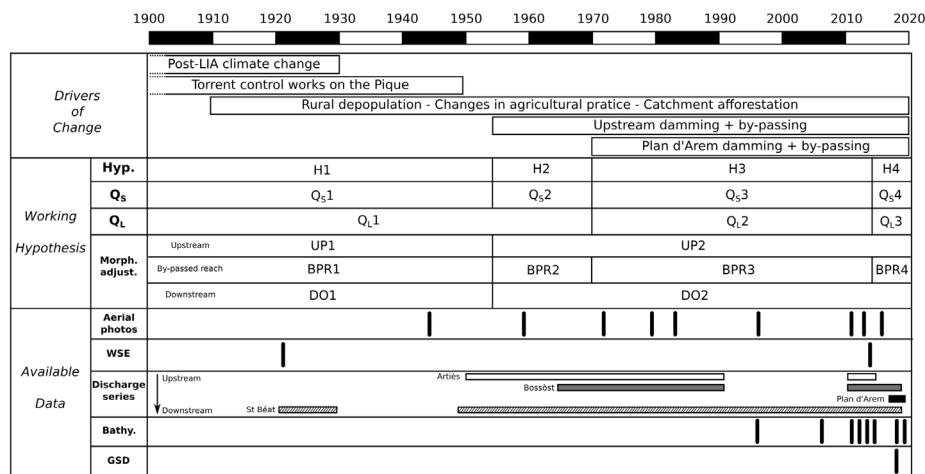
Figure 1. Chronology of drivers, expected changes in **Q<sub>s</sub>**, **Q<sub>L</sub>**, and river morphology, and available datasets (Boutault, 2020). WSE: Water surface elevation. Bathy.: Bathymetry of the Plan d'Arem lake. GSD: Grain size distribution.
